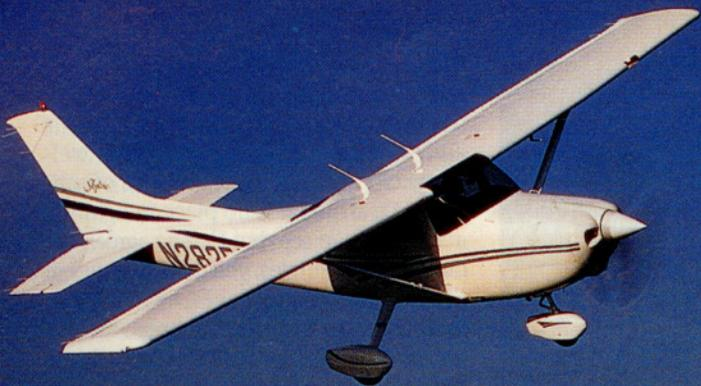
concerns. Preflighting the 182 involves taking fuel samples from five drain points in each of the wings. Two more sump drains are located on the belly. The wing tanks are of the wet-wing design, whereas most previous 182s had rubber fuel cells.
